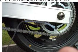
Step 4 – Routing the oil tube
