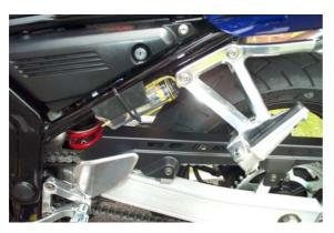
The first job, when fitting your Scotoiler is to decide where to place the oil reservoir, there are a number of different possible locations where people place them from under the seat to attaching them to the rear mudguard. For convenience sake, and to make it easier to keep an eye on the oil level I install mine on the frame, just forward of the rear foot hanger on the left hand side of the
