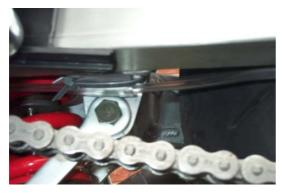
the oil tube is clear of the chain I secure the other clear plastic holder (hence the reason for cutting the first one in two) to the underside of the swingarm brace with tie wraps, and then route the tube through that. Once you are happy with the routing trim the oil tube to the required length and attach it to the underside of the oil reservoir. When trimming the oil tube
