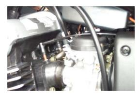
nipple, then install one end of the vacuum tubing (the thin black one) onto the connector. Anyone who has performed the modification that involves linking the carburetors together will need to split one of the hoses linking the carburetors and use the white 't' piece to connect up the vacuum pipe.
