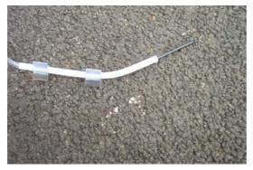
you will need to drill through the 'wings' on the holders and through the underside of the swing arm, then secure the whole assembly with self tapping screws (the whole job is easier if you use a drill bit half a millimeter smaller than the self tapping screws.
