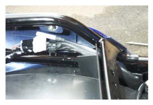
The only part of the Scotoiler unit that now needs fitting is the air tube / air filter pipe. Care should be take when placing this as the last thing you want is for water to be able to get into the tube as this would intern contaminate the oil. My preferred location for the air tube / filter is to actually place it inside the underseat storage space, tucked in to one side so that it will not get
