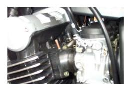
between the carburetors and the cylinder heads. For the sake of convenience I used the balancing nipple for cylinder number one (the left most cylinder as you ride the bike). Remove the black cap that covers the bleed nipple and then insert the black vacuum connector supplied with the Scotoiler onto the
